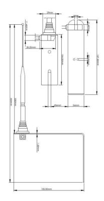
5/8 Wave multiband colinear antenna that can easily be wall mounted.
